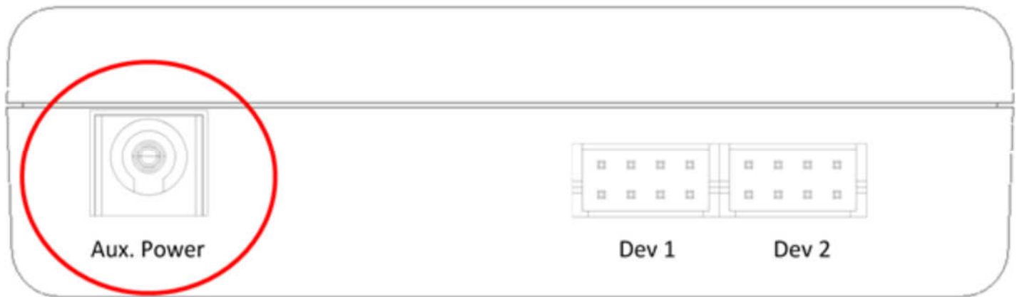
Figure 15 – Connecting external / auxiliary power
